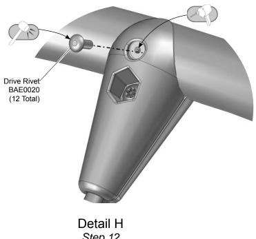
Step 12 Secure the connectors to the support ring.
