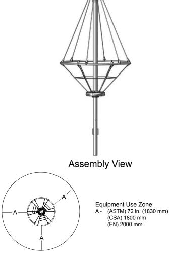
Refer to the Elevation View for the specific Critical Fall Height for the component.
