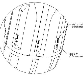
S 3/8" x 1-3/4" Button Head Bolt 3/8" x 1-3/4" Button Head Bolt Sutton Head Bolt Button Head Bolt Sutton Head Bolt Figure 1.5 SUPPORT BRACKET
